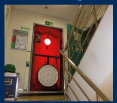
Problem: In the event of a fire or process incident offshore, Temporary Refuges (TRs) form a last line of defence to shelter and protect personnel at muster, by limiting as far as possible the ingress of gas or smoke into the refuge. Integrity is affected over time by degradation of ventilation dampers, door seals, module fabric and utility penetrations, leading to excessive leakage and the TR becoming impaired during an incident.
