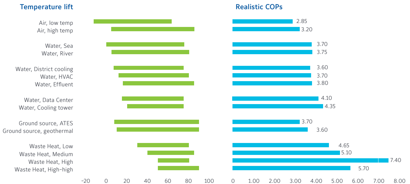
Figure 9. Different HP heat sources and related COPs.
